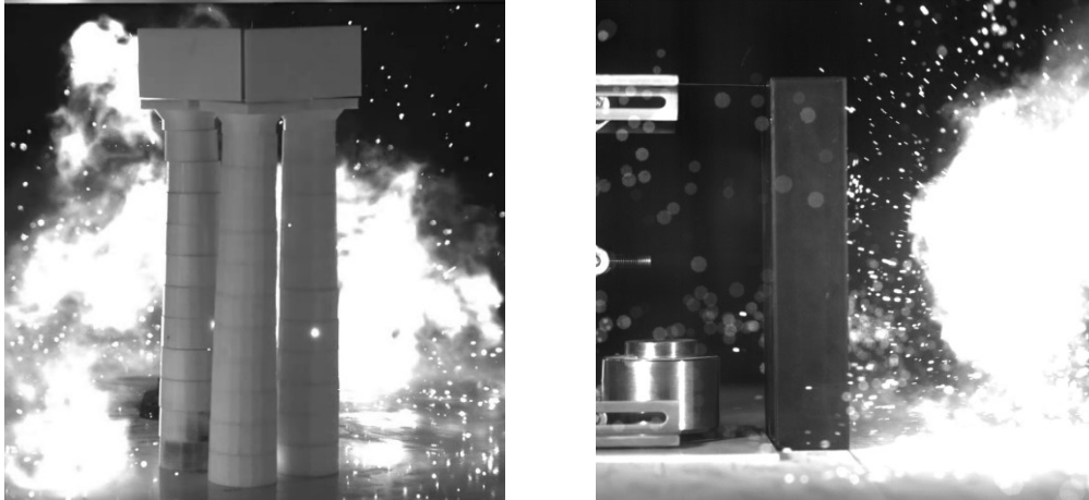
Fig. 5: Models (rocking structures) subjected to the fast-dynamic excitations arising from the denotation of an exploding wire.
